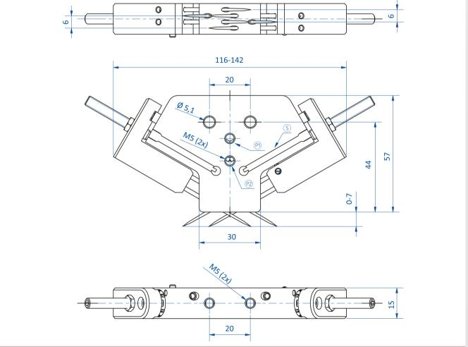
🕲 = Bore holes M5 for central extraction of needles 🔞 = Bore hole M5 for central retraction of needles 🔞 = Sensor slot
